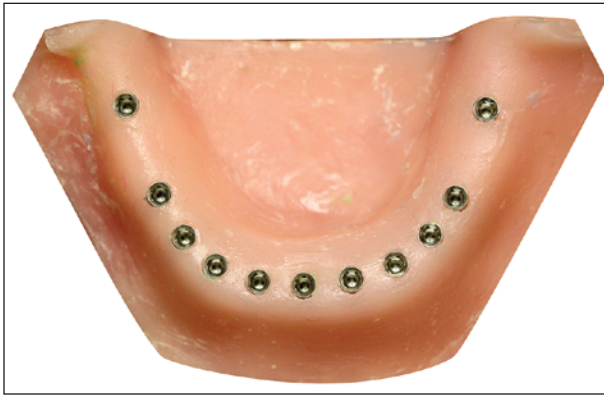
Fig 1 Acrylic resin test model and 3-mm gingival analog with 11 dental implants placed approximating tooth arrangements (central incisor, lateral incisor, canine, first premolar, second premolar, molar).
