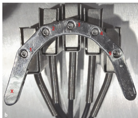
Fig 14 Comparison of experimentally-measured vs. predicted vertical forces on 4 (a) or 5 (b) implants supporting titanium bars loaded at the location of the 'X' in each figure. Predicted forces came from the Skalak model (Bench-top loading system designed and built by Mr Steve Hurson, Nobel Biocare USA).
