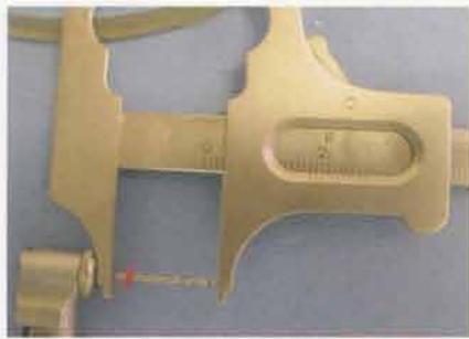
Figure 5 —Proper pilot hole depth is measured using an endodontic rubber stopper.
